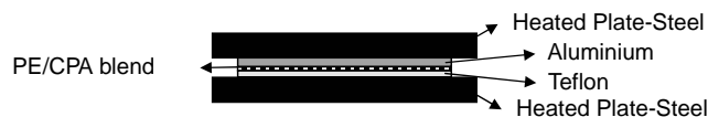
Fig. 1. Schematic drawing of the assembly used to obtain the compression moulded films. In the picture the case is reported where two different rigid sheets (teflon and aluminium) are used as moulding materials.
